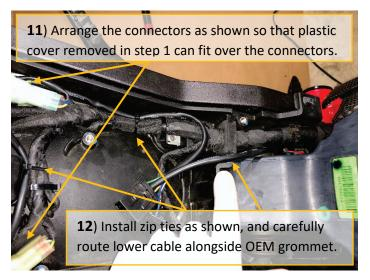
**13**) Reinstall plastic cover, and make sure all three harnesses pass underneath relief area as shown and fasten the cover.
